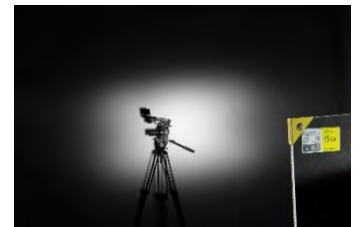
Hexagonal domed 33 mm Convex, Soft elliptic reflection with “cucoloris” effect depending of the distances
