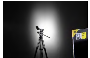
Hexagonal domed 33 mm Concave, Soft elliptic reflection with “cucoloris” effect depending of the distances
