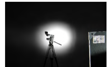
Shiny hexagonal domed 17mm Concave, Hard elliptic reflection with “cucoloris” effects depending on the distances
