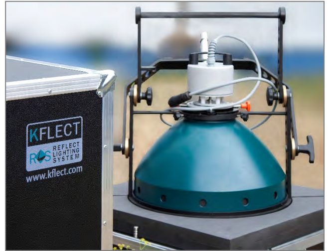
K-CASE 40 (K-BEAM on top of the cover, ballast, cables and bulbs are under the cover)
