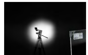
Shiny hexagonal domed 17 mm Convex, Hard elliptic reflection with “cucoloris” effects depending on the distances.
