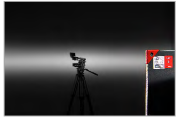
Narrow ripped / Hard linear reflection, helps creating a narrow lighted zone
